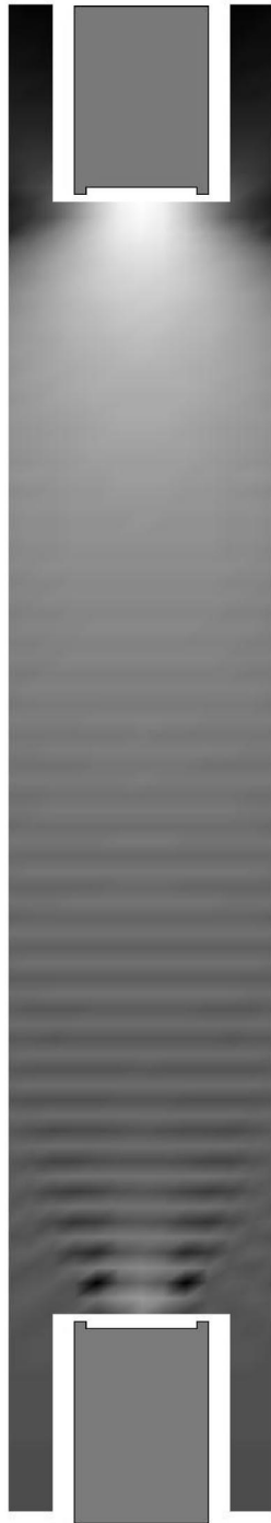
FIG. 8. The sound field between the two LS1 microphones, 20 cm apart in a free-field reciprocity setup at 20 kHz. The dark zones indicate minimum values, and the bright zones indicate the maximum values of the sound pressure.
